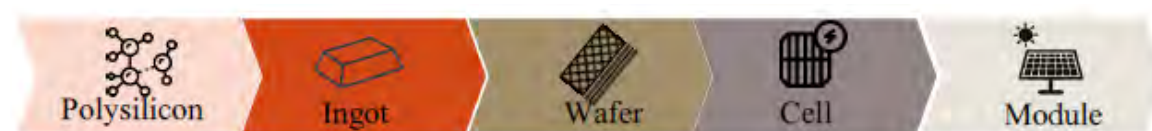
Figure 21: Schematic of c-Si PV module supply chain
